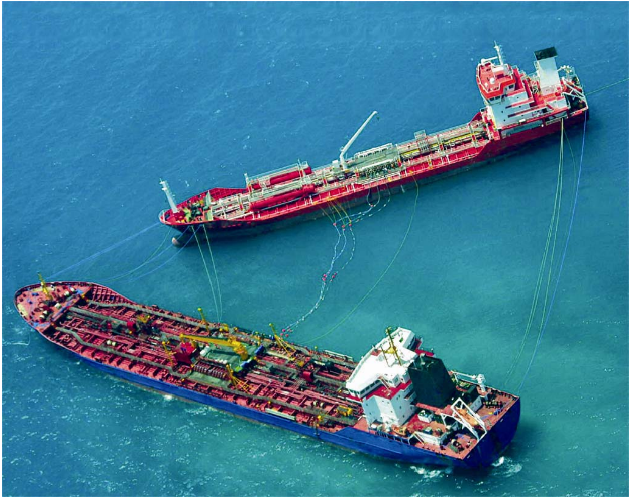
The T&T BISSO salvage team performs a ship-to-ship transfer of ethanol to lighten the tanker that ran aground.
