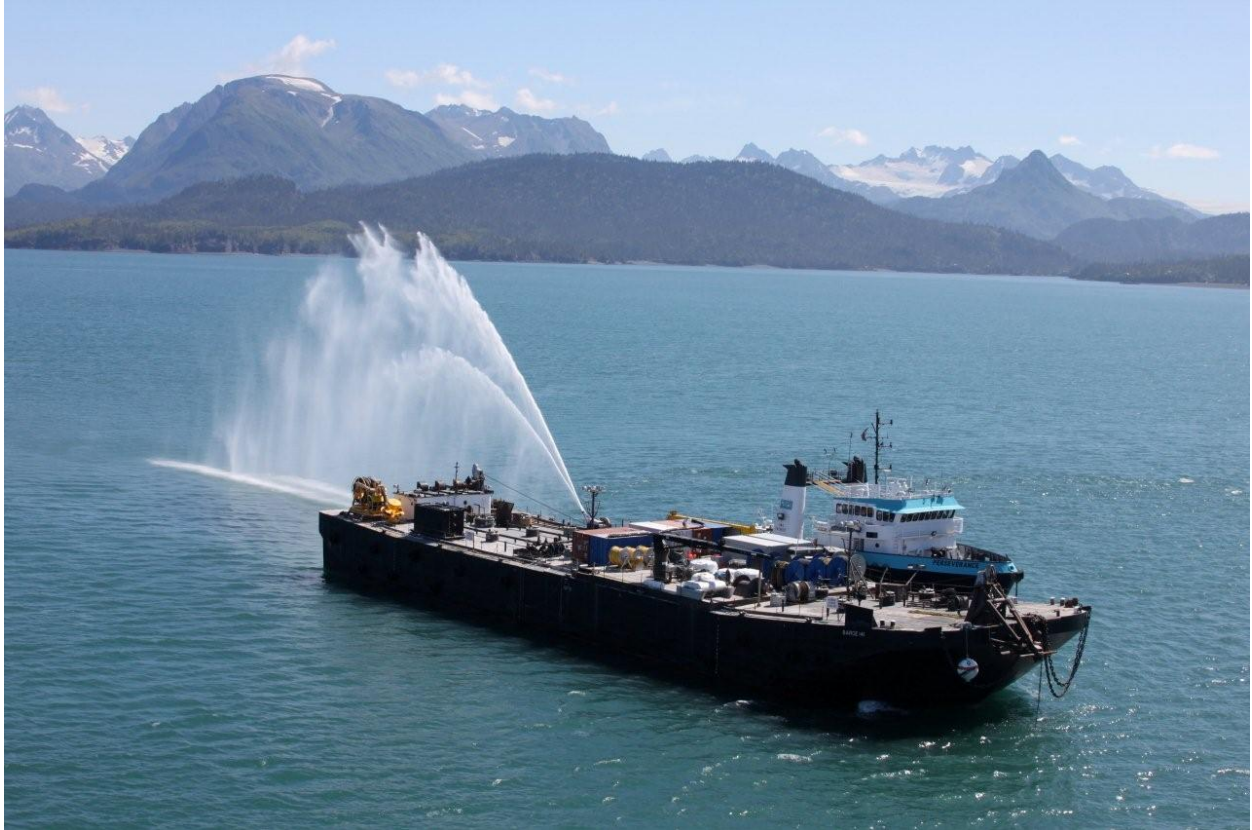
T&T BISSO RESPONSE displays its marine firefighting capabilities during equipment exercises in Kachemak Bay in Alaska. The TT-600 Fire Pump System has a capacity of 2,650 gpm, weighs 5,000 pounds and has a throw distance of 300 feet.
