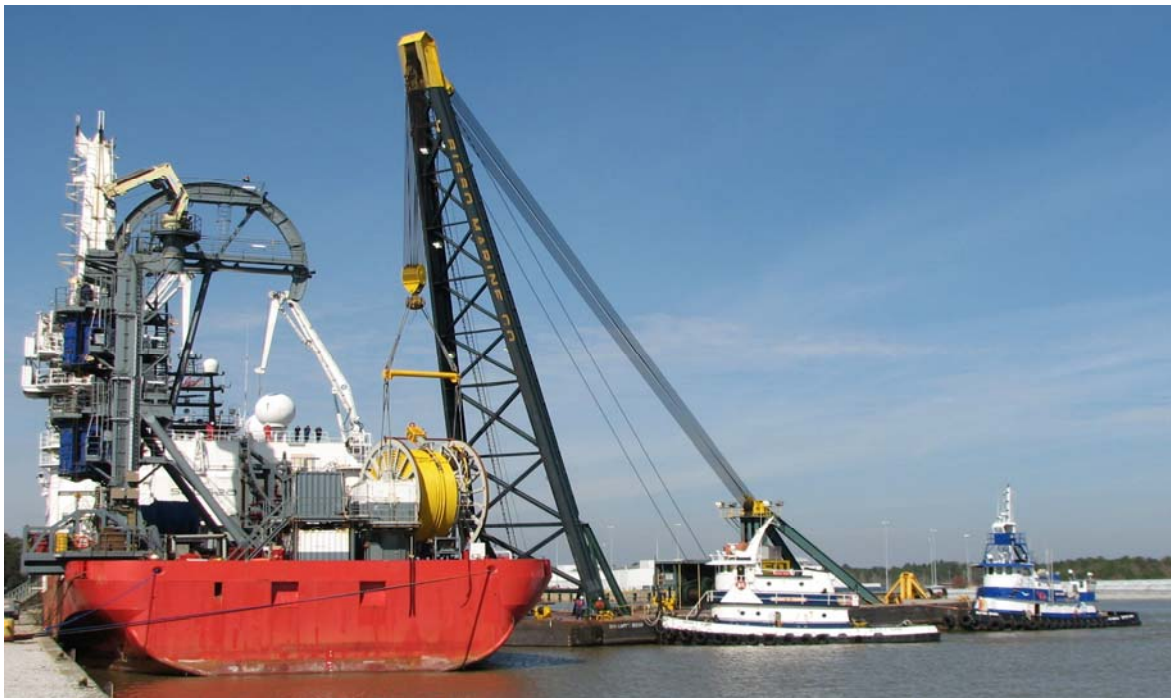
The D/B CAPPY BISSO loads a 281-ton umbilical reel from shore to vessel.
